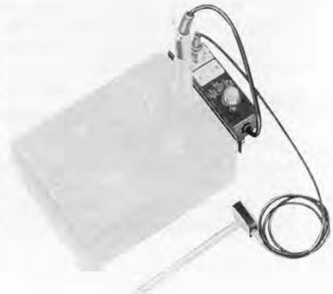
Figure 1. View of the Vibration Pickup System attached to the Type 1551-B Sound-Level Meter.
